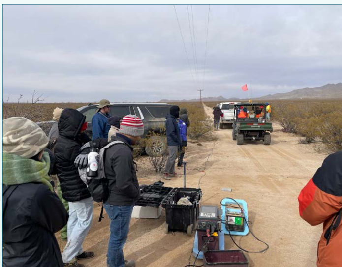
Figure 4. We conducted 2D ground-penetrating radar (GPR) surveys using the Sensors & Software NOGGIN 250 MHz system (left). On the same line, we undertook gravity and magnetic (middle) measurements. In addition, we used the Geometrics 64-channel Stratavisor system (which has been our educational workhorse for 20 years) as well as the Earthscope continuously recording 3C nodes and Dawson's vertical geophone nodes.
