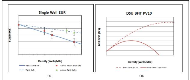
Figure 14a, b: The average EUR trend of Tank Developed Spraberry Shale wells is elevated relative to its Non-Tank Developed peers at comparable density. The shallower degradation trend in Tank Developed wells means that the DSU can support a greater number of wells at a considerable value multiple as compared to a Non-Tank Development regime (14b).
