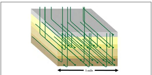
Figure 1: Example of challenging 3D horizontal development in multiple stacked pay horizons in a one mile drilling unit. Green lines are wellbores drilled from North and South in multiple formations.
