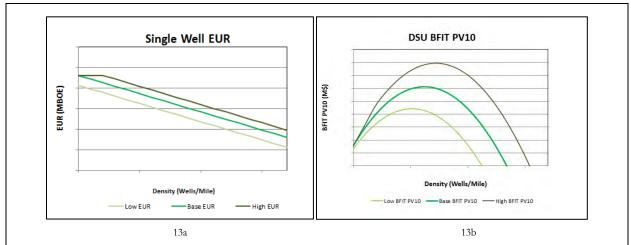
Figure 13a, b: With sufficient density tests, EUR can be expressed as a function of development density. Plotting average PV10 for wells at a given density allows the operator to understand the value ramification at scale. Figure b shows the DSU level cumulative PV10 across densities. The peak of this parabola corresponds to the density that maximizes the value of a drilling unit.
