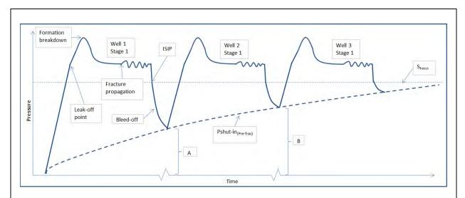
Figure 12: Schematic illustrating the following concept: Tank Development adds energy to the reservoir system faster than it can dissipate, resulting in greater number of fracture initiations in each subsequent completion, and thus greater near-wellbore complexity. Starting points A and B are higher than the first well's initial shut-in pressure (pre-frac), which translates to greater event generation and capital efficiency.
