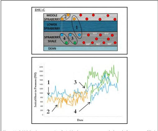
Figure 11: Initial shut-in pressures (pre-frac) rising between stages towards the end of a sequence of Tank Developed wells on the west side of DSU-C.
