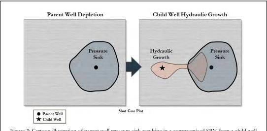
Figure 3: Cartoon illustration of parent well pressure sink resulting in a compromised SRV from a child well
