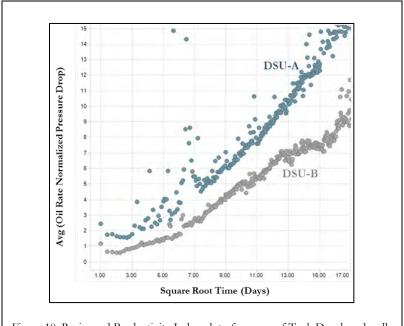
Figure 10: Reciprocal Productivity Index plot of average of Tank Developed wells (DSU-B completed at 16 wells/mile) compared to Non-Tank Developed wells (DSU-A completed at 10 wells/mile).
