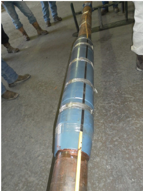
Figure 3 – Picture of one (of 37) ball drop valve used in the project.
