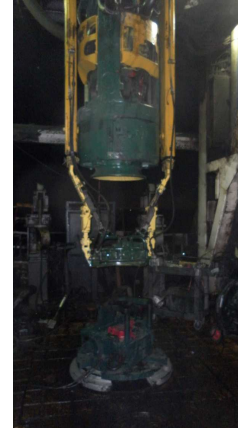
Fig. 10. The CRT is hanging above the rotary table.
