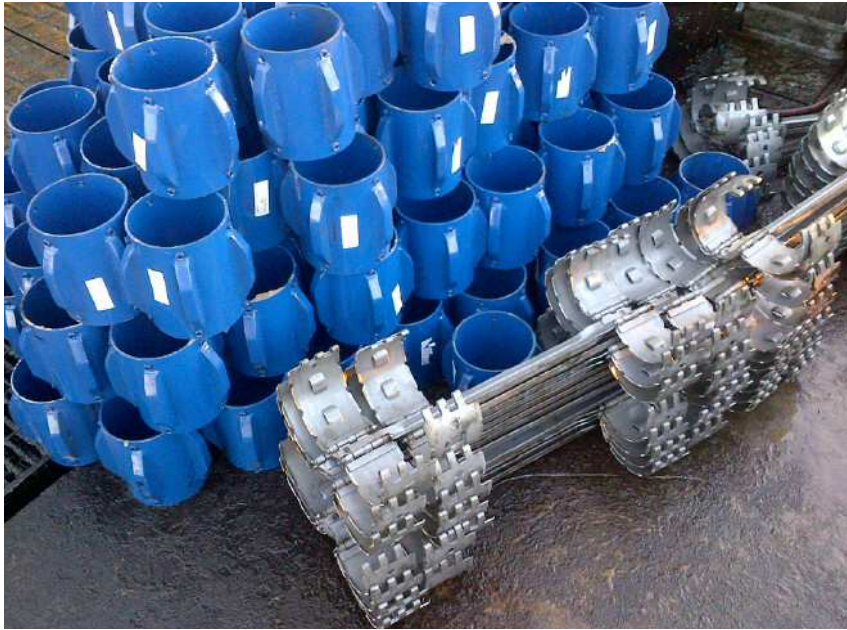
Figure 6 – Centralizers and cross coupling clamps are stacked on the rig floor.
