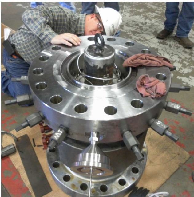
Fig. 9. Drilling Superintendent inspects the modified wellhead during the dry stack up of wellhead components at service company's facility.
