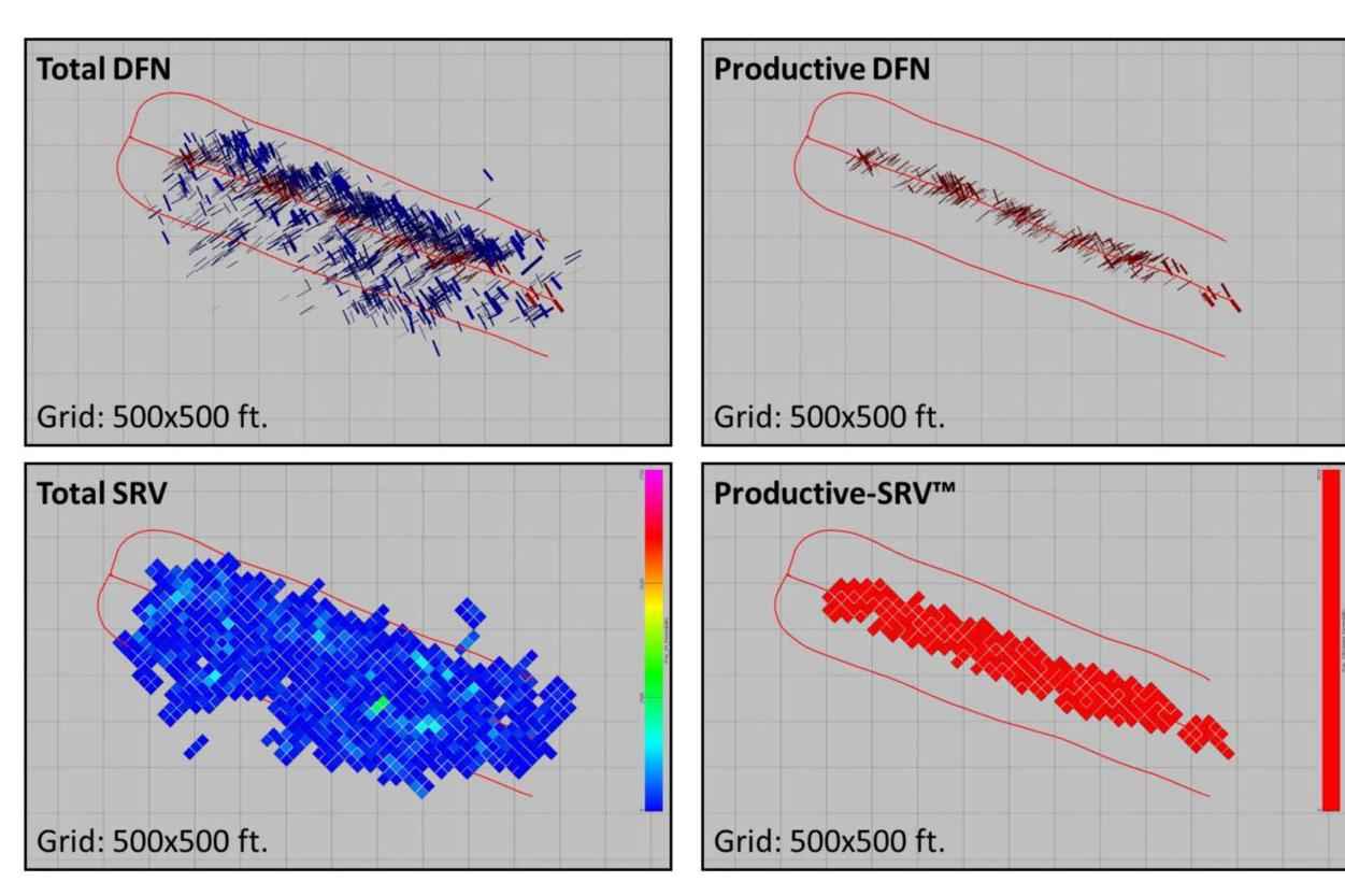
Wellbore spacing may be slightly reduced in order to provide a well-connected propped fracture network without undrained parts between wellbores leaving resources behind.
