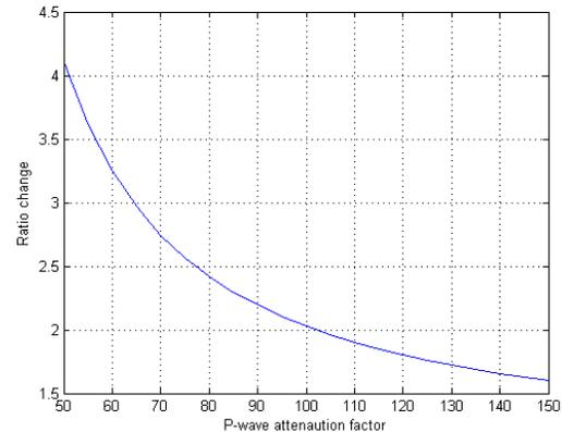
Figure 1 Ratio of ratios of P-to-S-wave relative amplitude in attenuating media ( $R/R_0$  in equation 1). Quality factor of S-waves is one half of the quality factor of P-waves, both P- and S-waves have similar dominant frequency of 100 Hz measured at 300 m distance from a receiver in homogeneous media with  $\alpha=4000$  m/s and  $\beta=2000$  m.
