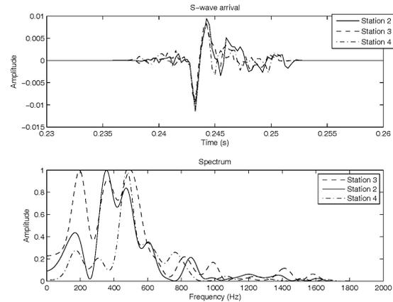
Figure 2 Particle velocity and their spectra for S-wave arrival on three geophones (station 2-4) with a sample rate of 0.250 ms in a nearly vertical borehole. The event is approximately 400 ft (121 m) away from the Station 2. The spectra were taken in a symmetrical window with a total length of 10.0 ms around the S-wave arrival with an additional 5.0 ms taper on either edges. Stations were separated by 50 ft (15 m).
