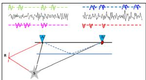
Figure 1: Wave Field Division (upper panel) and the geometry of receivers and model. Wave traces on the top-left and top-right are divided three parts of the wavefield at receiver A and B, respectively. Two receivers are placed on surface (Black Line). A reflector (Solid blue line) is located below the surface. S and R denote a source and a scatter, respectively.
