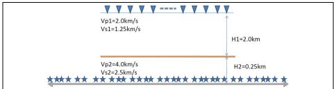
Figure 2: Setup of the numerical experiment. One flat reflector is located at the depth of 2.0km. 101 receivers are placed on surface with a uniform spacing of 50m. Source are randomly distributed at a depth of 2.25km. Constant P and S wave velocities for the upper and lower layers are given as Vp1, Vs1, Vp2 and Vs2, respectively.
