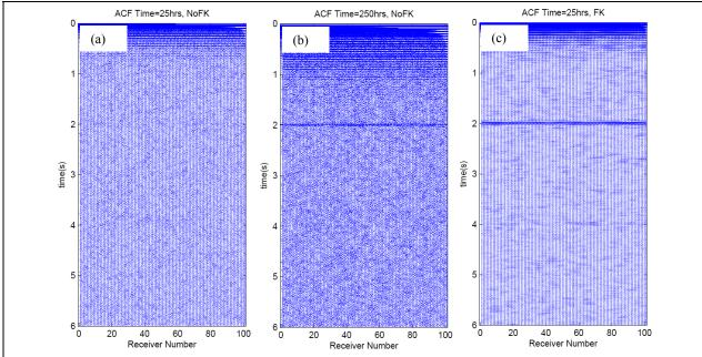
Figure 3: Summation of auto-correlation functions for different time length: (a) 25 hours; (b) 250 hours; and (c) 25 hours of data with FK filter applied before auto-correlation. The passband of the FK filter is (-0.05 -0.025 0.025 0.05)s/km. The horizontal bright spot is corresponding to the reflecor shown in the Figure 2. Every one hour of data consists of 4 time segments.
