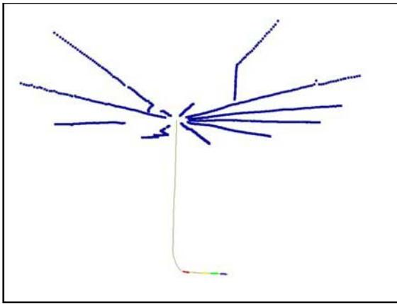
Figure 2: Map view of the relative locations of the 140 strongest events induced in Stage 5. Some events off applied to origin times. The 100 strongest (best of the main trend are "false positives" due to the signal-to-noise ratio) events form a simple trend with cross-correlation side lobes. an approximate 80° azimuth.
