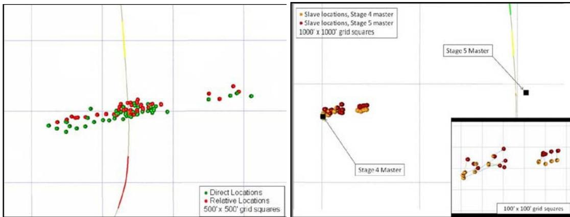
Figure 6: Map view of located events for five stages using matched filter technique. Event color corresponds to treated wellbore interval.
