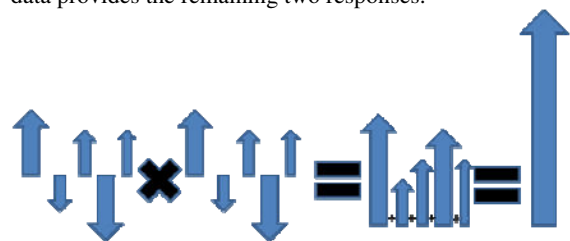
Figure 1: Illustration of noise enhancement by cross-correlation of similar waveforms.
