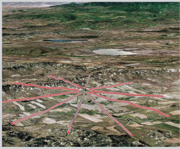
Temporary FracStar® array design depicting sensor placement.
