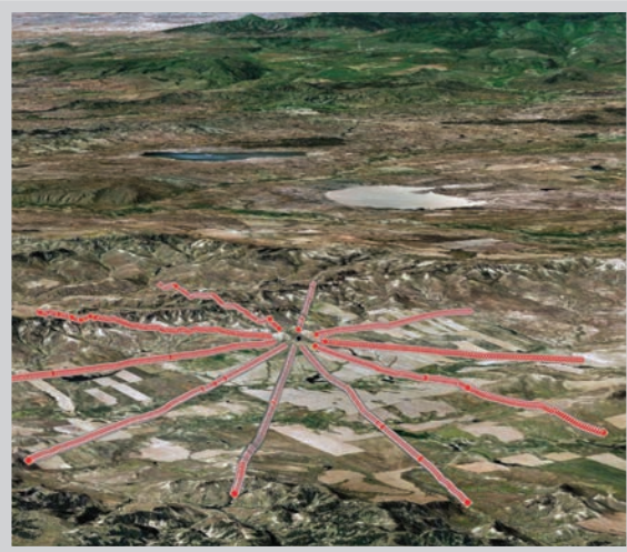
Temporary FracStar® array design depicting sensor placement.
