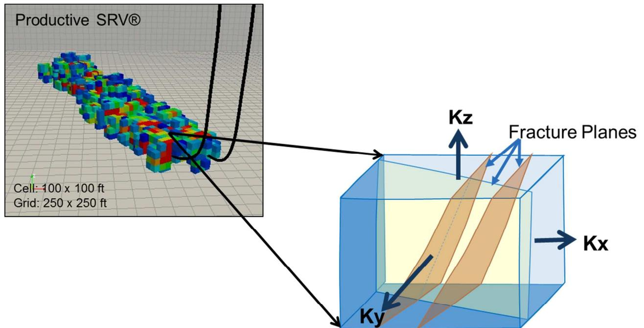
Figure 1: Computing permeability tensor
