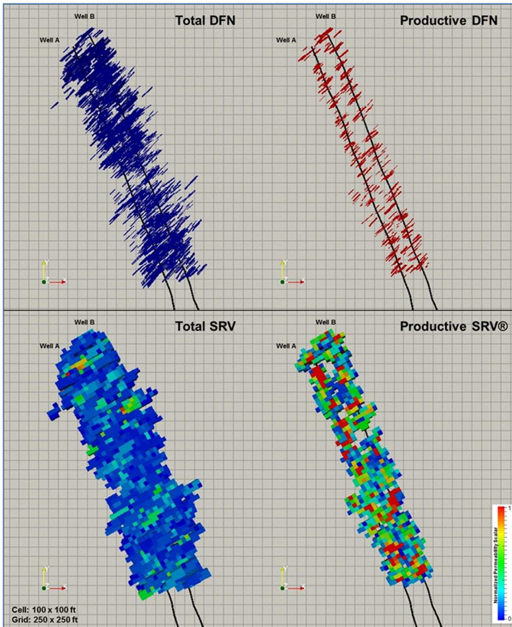
Figure 2: DFN and P-DFN Models (Top); corresponding SRV and P-SRV models (bottom)
