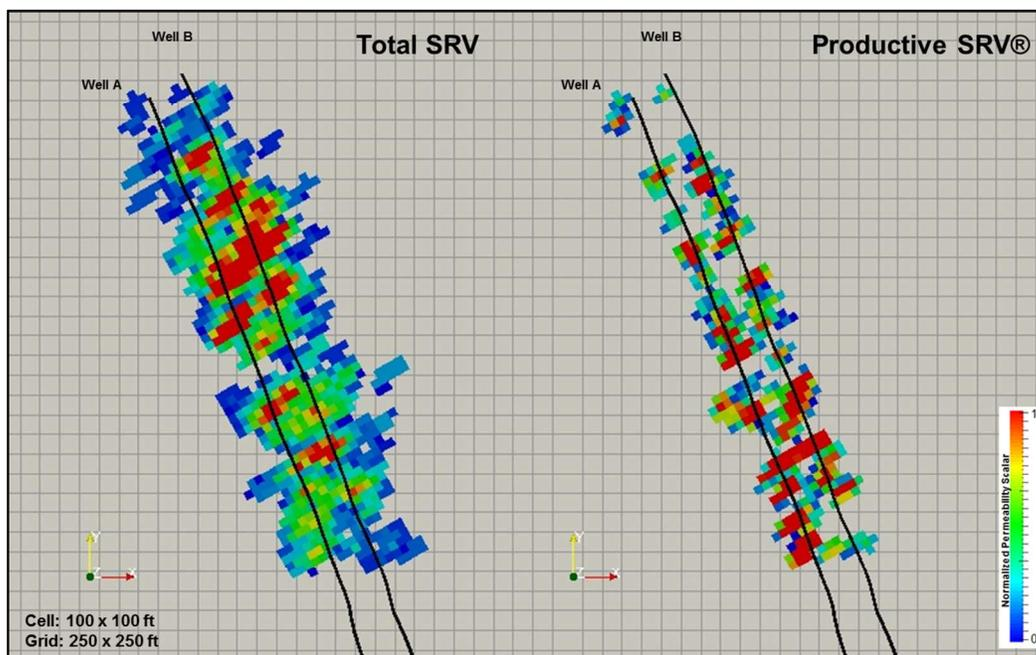
Figure 3: Depth Slice of SRV (left) and P-SRV (right) @ 200ft TVD below the wellbore
