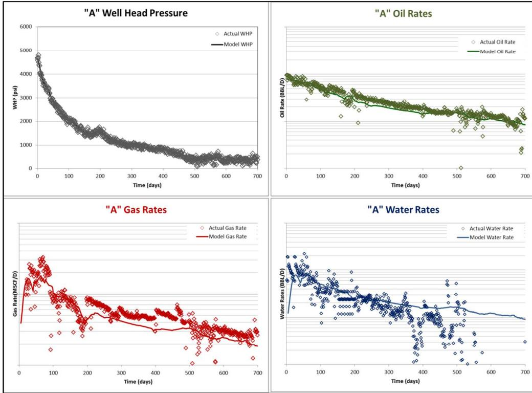
Figure 6: Production History-Matching/Calibration of Model (solid lines) with Actual Production Data (dots) From Well A
