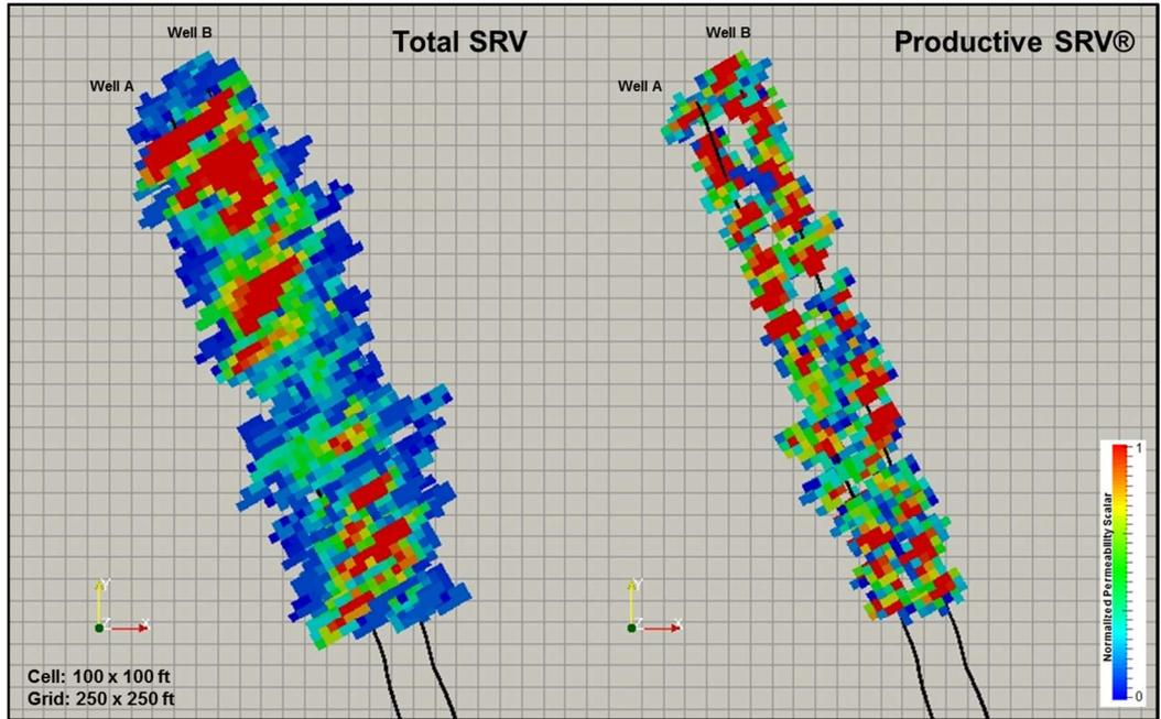
Figure 1: Depth Slice of SRV (left) and P-SRV (right) @ 200ft TVD above the wellbore
