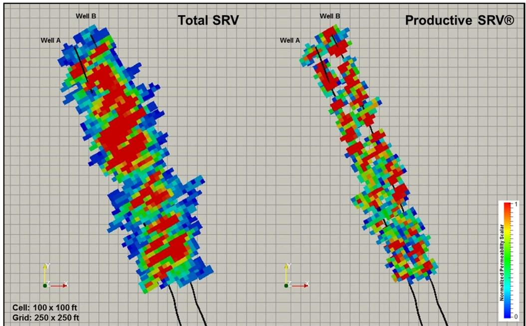
Figure 2: Depth Slice of SRV (left) and P-SRV (right) @ wellbore TVD
