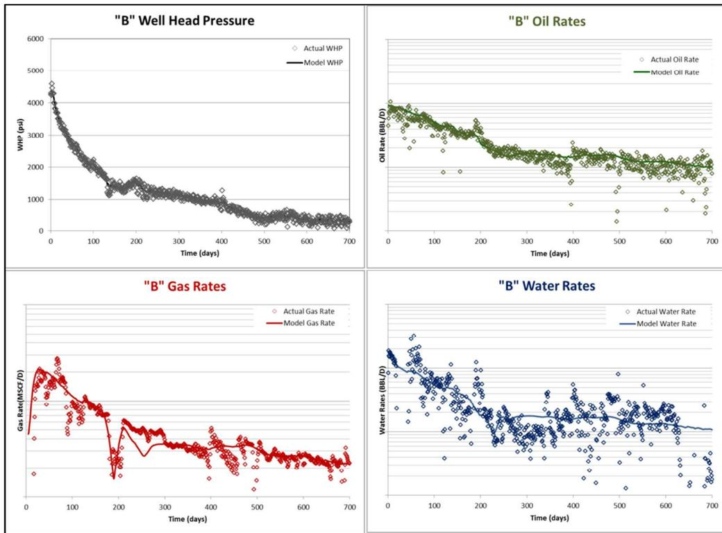
Figure 7: Production History-Matching/Calibration of Model (solid lines) with Actual Production Data (dots) From Well B
