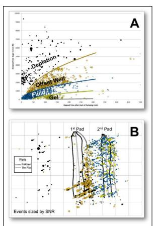
Figure 2: A - Plot of microseismicity sized by signal to noise ratio (SNR) showing classification of events associated with slickwater (Fluid, blue), the more viscous gel (Gel, yellow), events occurring on offset wells (Offset Well, orange), and events occurring on depleted wells (Depletion, black). B – Map showing locations of events shown in A using the same color scheme.
