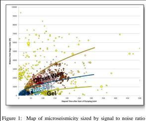
Figure 1: Map of microsetsmicity sized by signal to noise ratio (*SNR*) showing classification of events using Ward's algorithm. X-axis is elapsed time after start of pumping (t) and Y-axis is distance from stage center (r).
