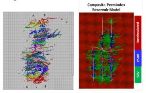
Figure 4: Left-Microseismic Data, Right-Composite Reservoir Model
