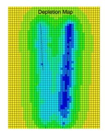
Figure 3: Pressure Depletion Map after 18 months of production
