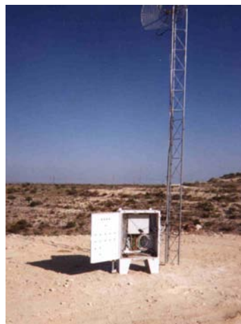
Figures show a PMM system monitoring a CO 2 injection into a hydrocarbon reservoir in West Texas.
