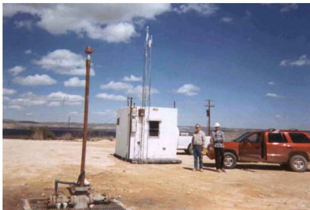
Figures show a PMM system monitoring a CO 2 injection into a hydrocarbon reservoir in West Texas.
